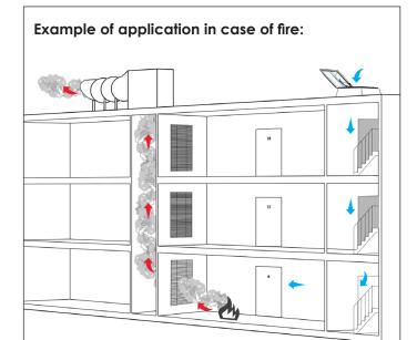
Damper opens and fan starts. The smoke and gas is drawn up and out via the exhaust duct.
